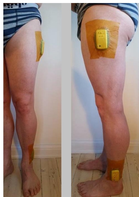
Figure 1: Wearable sensors placement on the leg attached with Ioban.
